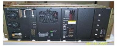
**Quantar Radio**: A Motorola radio intended for use as a base station, either as a radio or as a repeater. It is capable of conventional analog as well as transmission and reception. Its output power is 125 watts.
